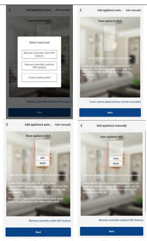
Reset the air conditioner (refer to the operation instructions in APP interface) and click -Next" to add home appliance automatically (Wi-Fi password shall be input). Or after setting and energizing the air conditioner, click -Add appliance manually" at the right upper corner to select the wireless network for controlling the device. Then confirm family Wi-Fi and arrange configuration.
