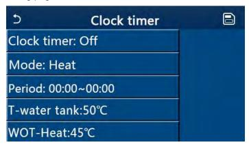
★ The option -Mode" is used to time the desired mode; -WOT-Heat" and -T-water tank" is used to set the corresponding water temperature; -Period" is used to for time setting. After that, by touching the -Save" icon, all settings will be saved.
