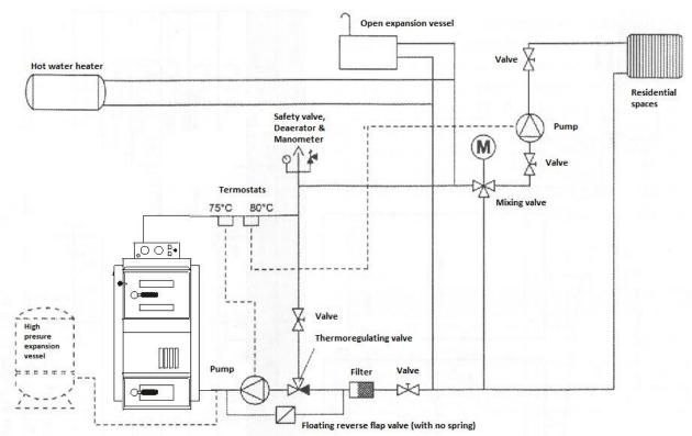
Boiler Installation/Connection with a Thermoregulating Valve
