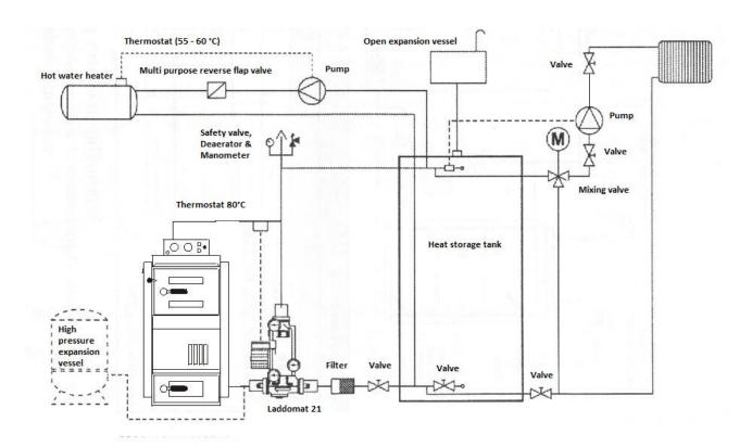
**Boiler Installation/Connection with a Heat Storage Tank**
